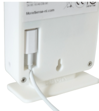
C-type side of the USB cable connected to the sensor
